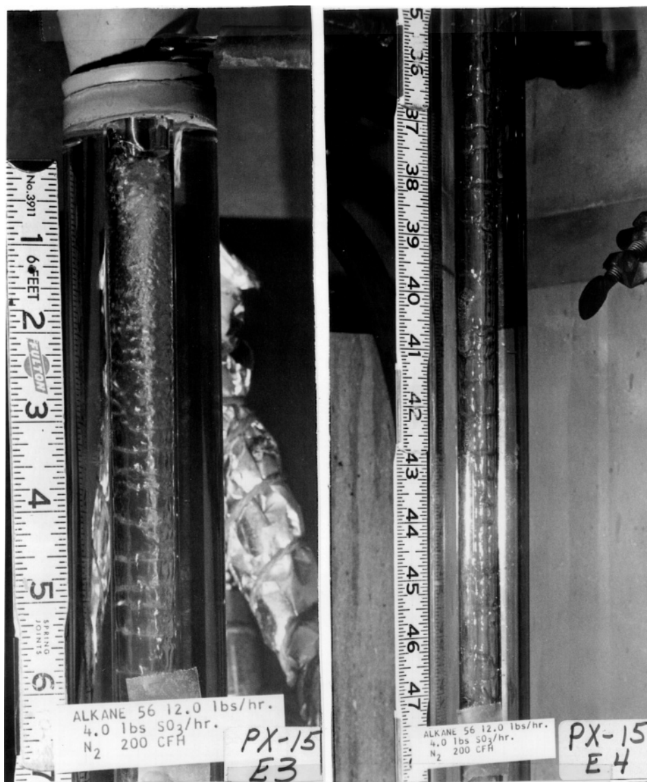
Figure 1. Composite of two photographs showing actual continuous \text{SO}_3 sulfonation of branched-chain detergent alkylate using 5% \text{SO}_3 in a nitrogen gas stream in a cooling jacketed 1.1 cm i.d. \times 122 cm glass reactor tube, alkylate flow 0.14 kg/(h \times mm circumference), and gas velocity of 28.3 m/s. (Left) Top of reactor. (Right) Bottom portion of the reactor. (Photographs courtesy of Rodger L. Peters.)
